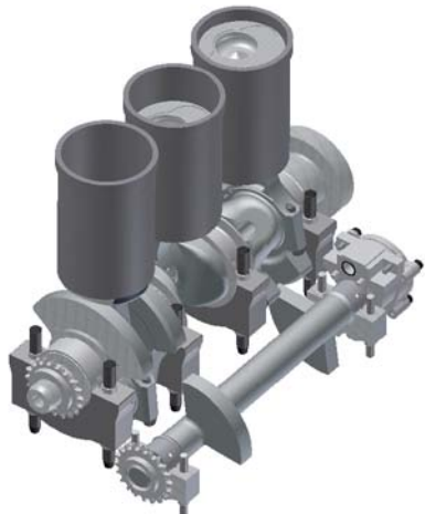
Figure 2: Crankcase Components including Oil Pump/Balancing Shaft
